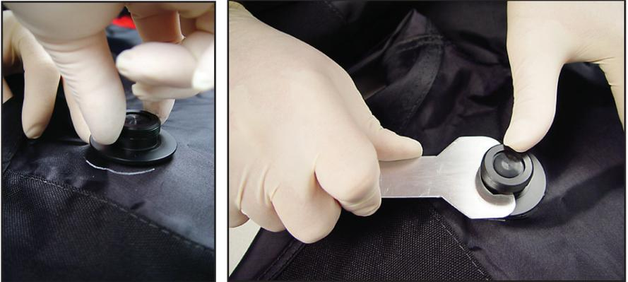
*After applying Aquaseal to the base of the valve (top left), work quickly to position the valve assembly in the desired direction within the suit and then press to seal the fabric on the base. Apply Aquaseal to the top seating surface, thread, then use the supplied wrench to hand-tighten valve.*
