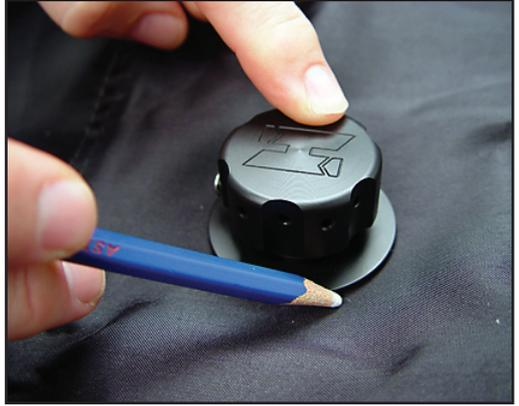
*Mark the location of the valve after carefully deciding on where you want to make the cut into the suit.*
