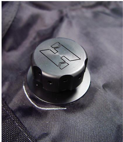
set screw to make sure that the external cap cannot be removed from the valve, gently tighten the set screw with an Allen wrench until the head almost touches the cap body. Test to ensure that the external cap is able to be loosened approximately two full turns and then stops. If the cap seems to bind, back the set screw out slightly until the movement is unimpeded. Use of the set screw is optional– however it can prevent accidental loss of the cap.
